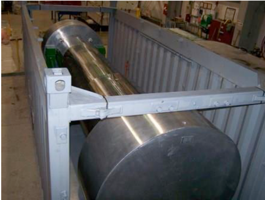
Fig. 2. NAC-LWT cask in a truck shipping container
